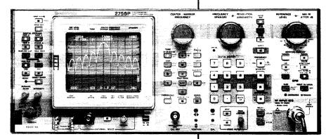
internal mixer, and to 325 GHz with external mixers such as Tek's WM490 Series, or the new WM780 Series (each WM780 Series mixer is indivually calibrated). Signal sensitivity is an impressive -134 dBm. The 2756P is optimized for use in baseband through millimeter-wave measurements, where the ability to identify and process signal frequencies and amplitudes over wide dynamic ranges with high accuracy is critical.
